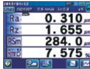
4-parameter display: four parameter measurement results
